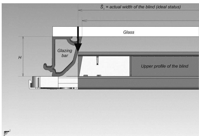
The ideal measurements of the blind are in the diagram. Such measurements can be taken by using the cut of the upper profile, the side board; by placing this aid on the glazing bar it is possible to state the point, the maximum possible width of the blind, and from this point the dimension of the same point on the opposite side is measured. This marking is always influenced by the form and size of the glazing bar of the window profile.
